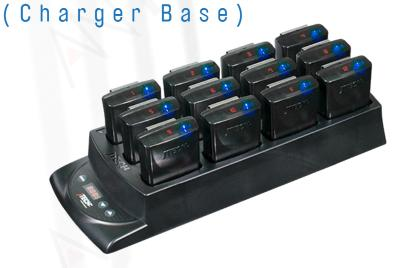
Model No of Slots Ratio Full Charge Dimension Weight CHRG-12 12 slots base 3 by 4 rows Approx. 4 hours 309mm 115mm 45mm Approx. 1.04kg
